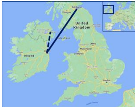
Figure 11. Exemplary flight route and profile of the design range mission EDI–DUB (Edinburgh, United Kingdom to Dublin, Ireland) (including the flight to the alternate BFS (Belfast) and a holding of 30 min)
