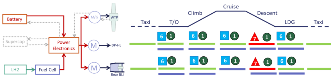
Figure 22: Energy management strategies for hybrid-electric architecture with fuel cell and batteries
