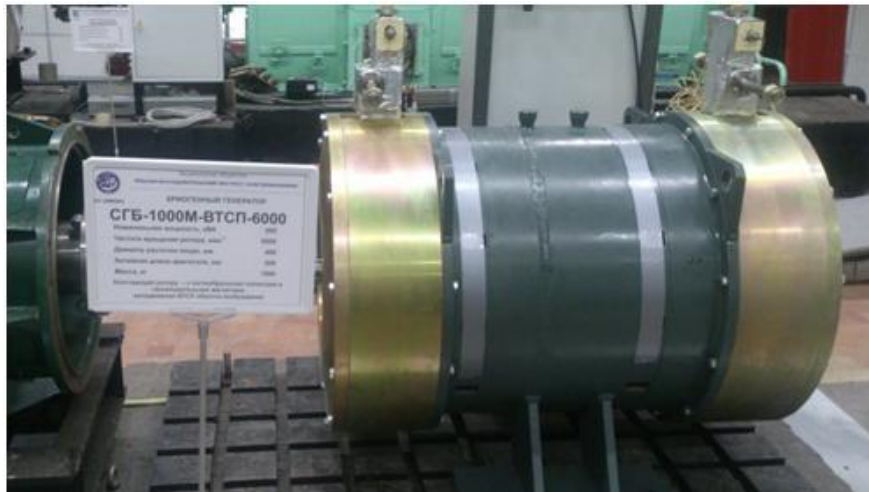
Figure 6.16: 960 kVA HTS generator with combine excitation
