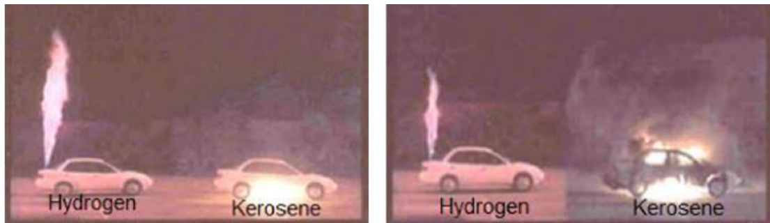
Figure 4.7: Comparison of hydrogen and kerosene fire done by the University of Miami (picture from [4.7])
