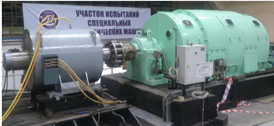
Figure 6.15: Comparison of 1MVA HTS generator and conventional one
