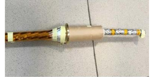
HTS-2G compact multilayer cable, outer Dia 20mm, 3kA@77K, 20kV insulation
