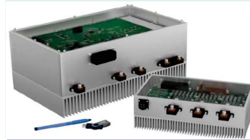
48V/12kW inverter with SiC (left) and GaN transistors (right)
