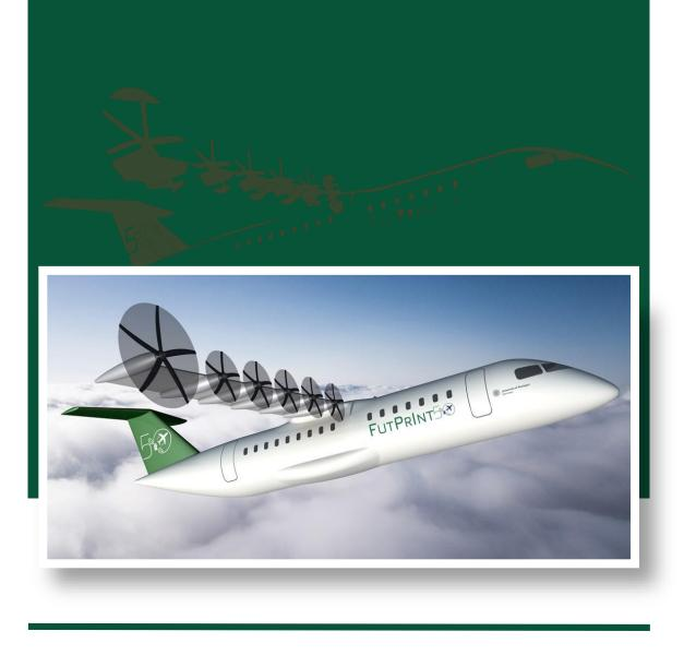
Figure 1: Distributed Propulsion Concept from FUTPRINT50 Project
