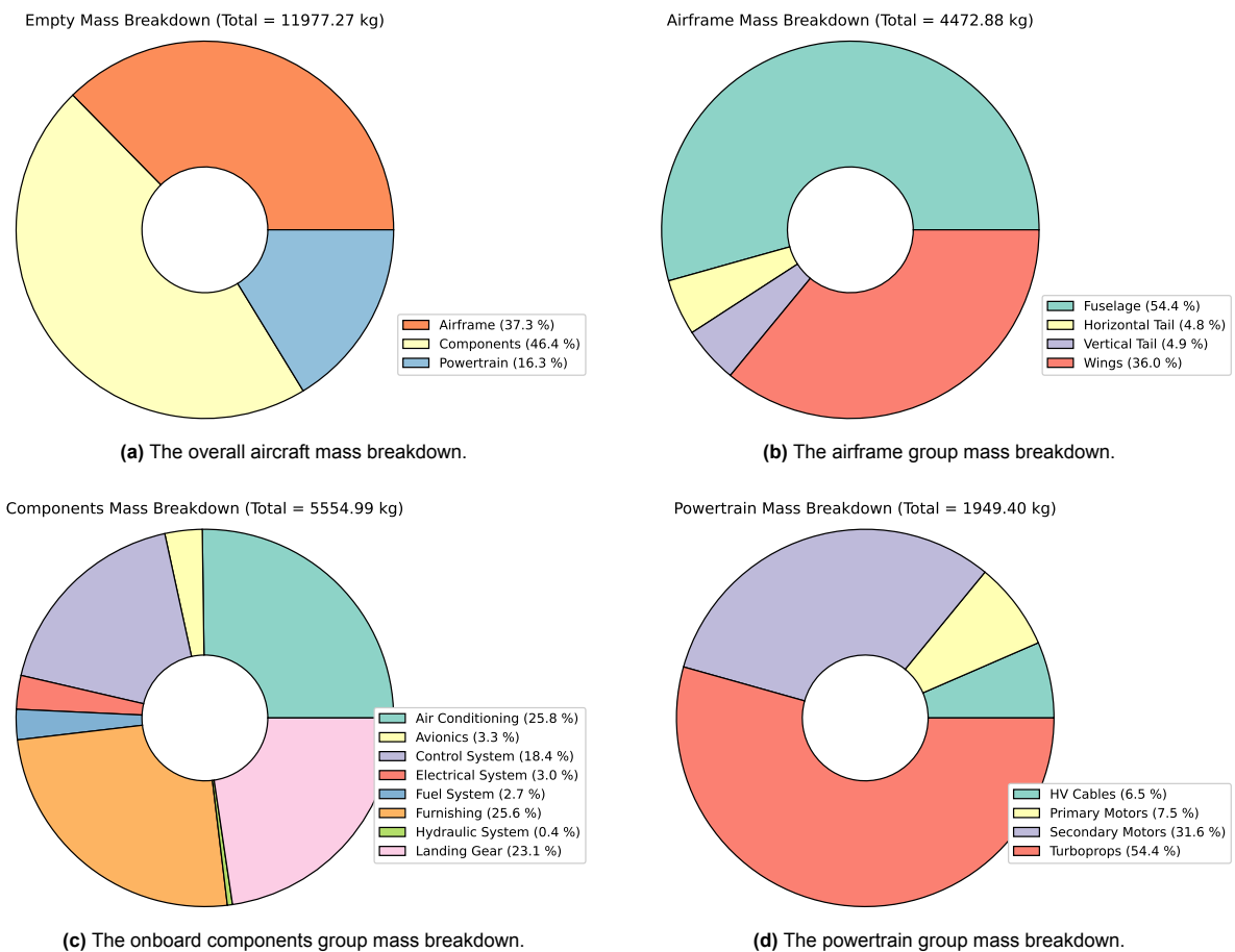
Figure 3.10: Plots containing the mass breakdown for the final aircraft configuration (will replace accordingly).
