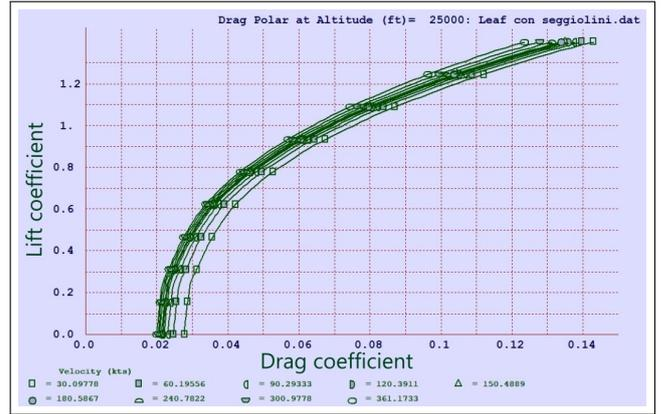
Figure 2: Polar aerodynamic diagram referred to the cruise phase.
